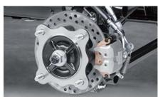
Rear Discs are 212mm with single 34mm piston caliper. Semi-metallic brake pads offer the right balance between braking power and long life.
