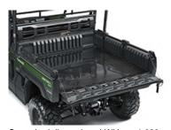
Cargo bed dimensions LWH are 1,089 mm x 1,363 mm x 279 mm in 3-person mode and a handy 560 mm x 1,363 x 279 mm in 6-person model, its long, flat design makes it easy to load from three sides. Cargo bed load capacity is 453 kg 3-person mode or 158 kg in 6-person mode.
