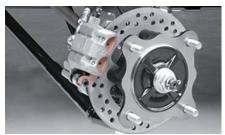
Front Discs are 212mm and gripped by two-piston (27mm) calipers.
