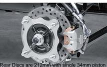
caliper. Semi-metallic brake pads offer the right balance between braking power and long life.
