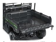
Cargo bed dimensions are 1,375 mm L x 1,355 mm W x 280 mm H. Its long, flat design makes it easy to load from three sides. Cargo bed load capacity is 453 kg.
